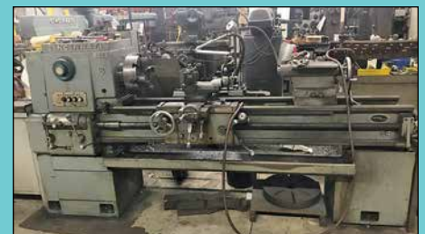
18" x 54" Cincinnati Tray Top Toolroom Lathe w/ Taper Attachment & 12" Chuck
