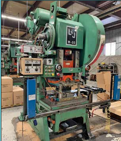
(16) L&J Back Geared and Flywheel Type OBI Presses Up To 100 Ton
